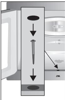
Slide the microwave into the cupboard. Open the door of the microwave. There is a round opening at the front middle for inserting a screw. Screw the microwave and cover the screw with the cap.
