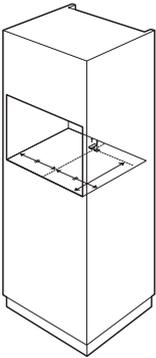
**Please note for the A2132HRVS:** first fit the support in the cupboard (see drawing). This support prevents the microwave from tilting forwards.
